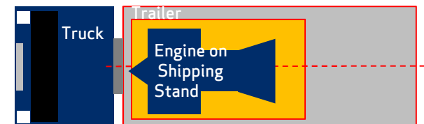
Shipping stand installed lengthwise and not protruding
